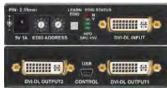
Lightware DA2DL EDID Manager + 1:2 Verteiler DVI DUAL LINK 330MHz
